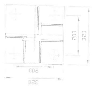
DETAIL AT - 'X' ANCHOR BOLT SETTING PLAN
